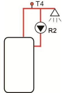
Trigger on conditions of temperature controlled DHW circuit pump (STAT): when tank temperature (upper temperature T3 is priority sensor) is 2°C higher than the preset switch-off temperature of this function (CYCF), DHW pump just can be triggered.
