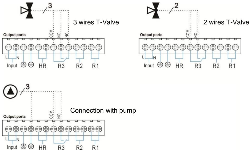
R3 connect with T-valve: (COM common terminal, NO always open terminal, NC always close terminal)
