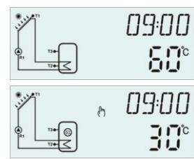
**i** **Note:** Manual heating is not a continuous heating process, it is triggered manually, and when the temperature reaches to the set point, the heating process is stopped. And manual heating function is stopped automatically.
